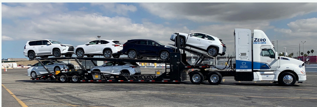
Toyota Logistics Services has put four hydrogen-powered fuel cell electric trucks into service for vehicle delivery in the Los Angeles metro area. These trucks are married up with trailers that can carry up to seven new Toyota/Lexus vehicles. Three of the zero-emission trucks are stationed at TLS’ Long Beach vehicle distribution center and haul imported vehicles, and one is at Union Pacific Railroad’s Mira Loma rail ramp and delivers North American produced vehicles.
